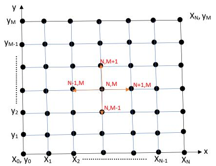
Let us divide the interval  $0 \le x \le 1$  into (N+1) equally spaced points.
